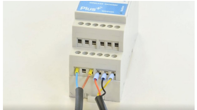
Wire Indication: Blue - GND; Brown - +24 VDC; Orange - Data+ (A); Black - GND; Yellow - Data - (B)
