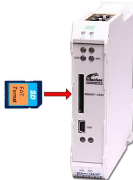
Figure 8: Insert SD card
