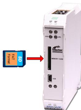
Figure 28: Insert SD card
