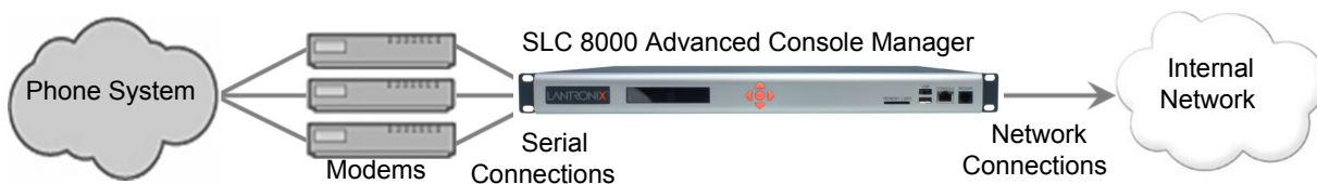
Figure 11-2 Remote Access Server
